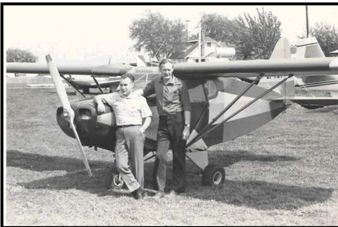
It was a home built put together by one of my friends R. Vanwoerden. The aircraft was a "Stits 65 Continental", (later converted with a 85 Continental). For this aircraft I was the "daring" test pilot.
